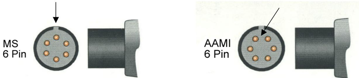
**Mechanical:** Six pins located equally spaced within a protective ½" circle rim that includes a keying slot. The pin nomenclature is not visible from the front thus the differentiation is whether the key is 'at the pin' or between two pins.
